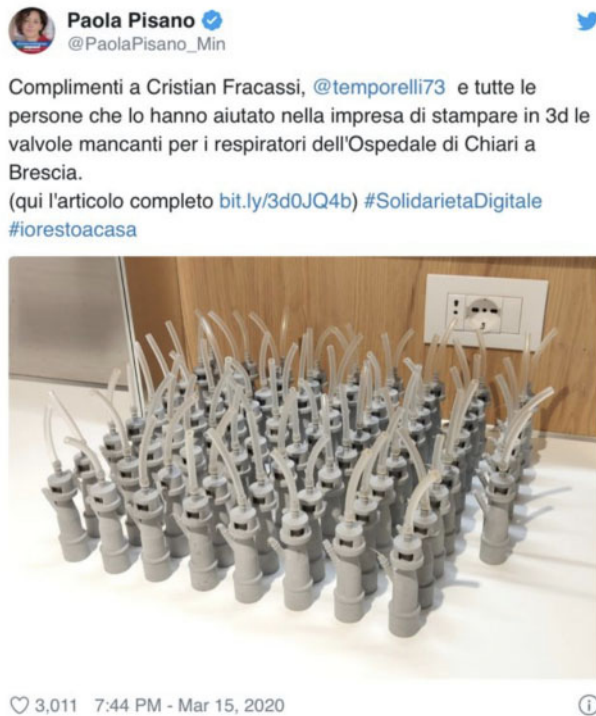
Figure 1. Tweet by Paola Pisano showing 3D printed valves for emergency ventilators during the COVID-19 crisis in 2020.
